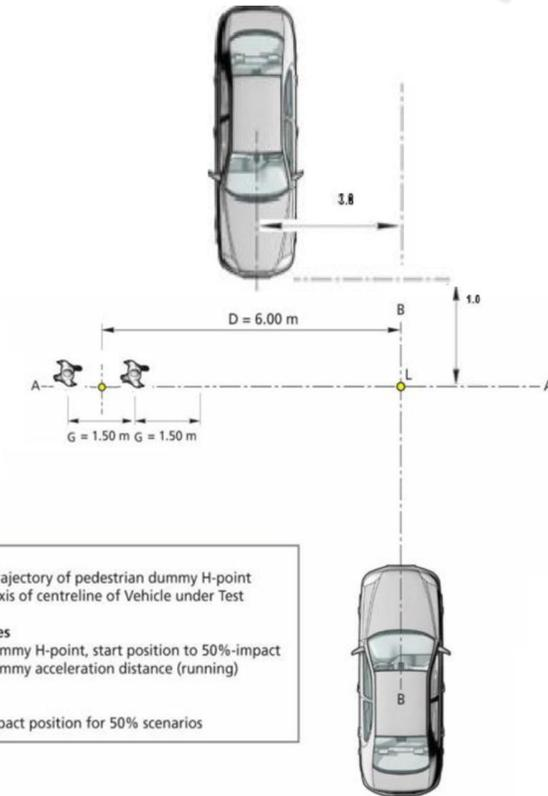
Theoretical example of a baseline CPFA injected with several robustness layers (multi-pedestrian, pedestrian appearance, clutter (stationary vehicle on adjacent lane)).
