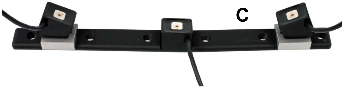
Figure 6. LEDs mounted on rib stiffeners
