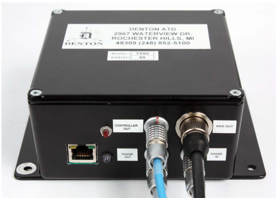
Figure 7. Trunk box (interface box)
