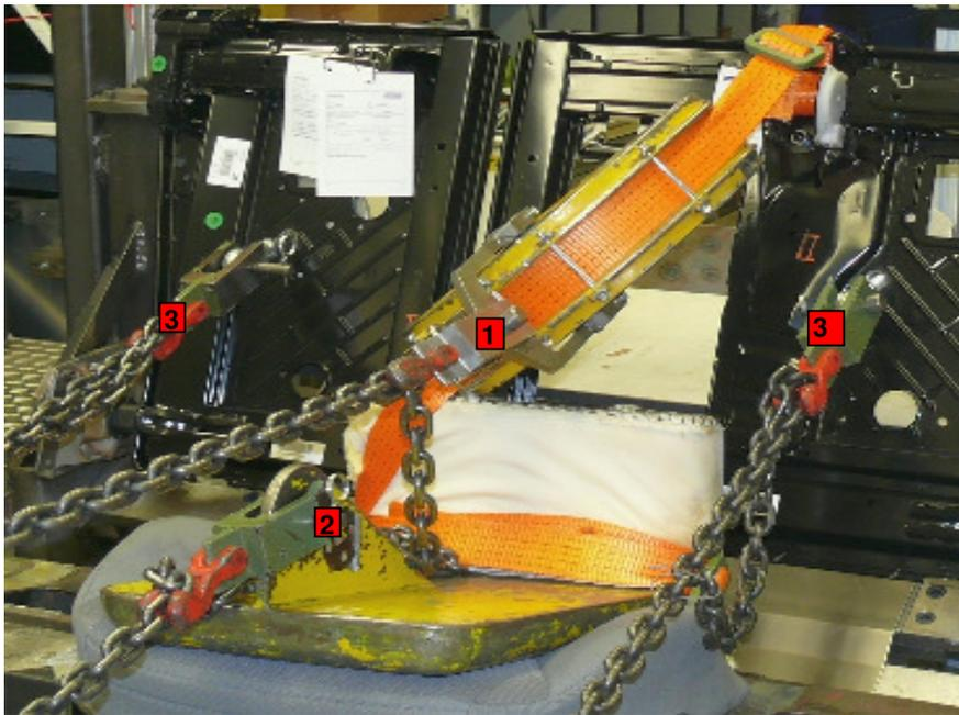
**For the center of gravity of the 60% part always use the outer position number**
